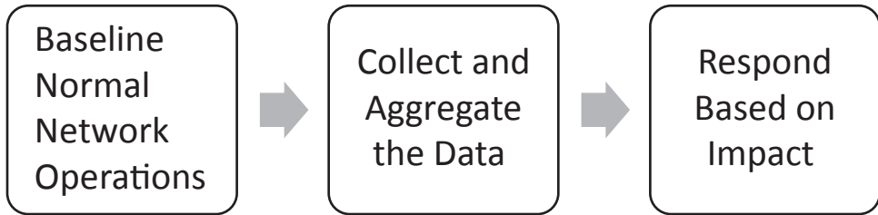
Figure 3-6. Strategy for detecting events, based on objectives of the anomalies and events subcategory of the NIST CSF
